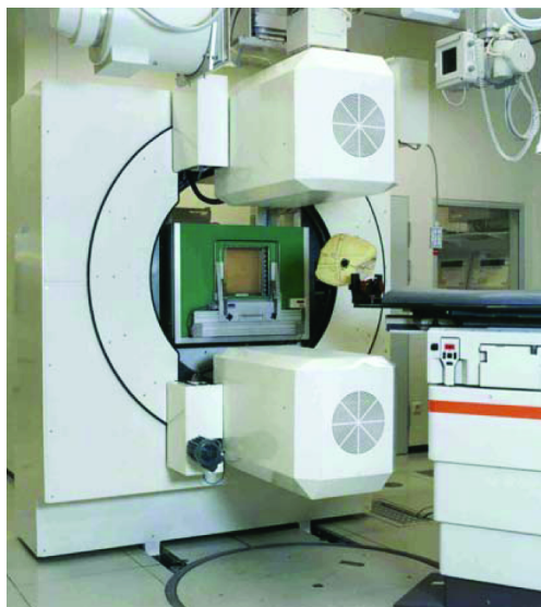
Figure 35. Picture of the PET camera used for the range monitoring at the GSI. Extracted from [Paro08]
